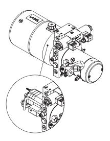
The W83D series power pack is designed for applications that need high pressure and larger flow, but use a low-power D.C. motor. The power pack uses a special manifold (W800553). All screw-in cartridge valves have been designed to be adjusted easily to service the power pack quickly. They still have the same dimensions and functions as the standard manifold (W800532).
